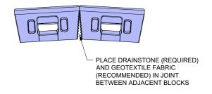
14 ft - 6 in (4.42 m) is the minimum radius for Novum blocks. It occurs when all of the blocks are placed tight together. A larger radius is required on the bottom row of a Novum Wall to account for the batter between courses of blocks and still provide enough space to construct the top row of blocks.
